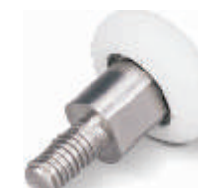
KT1600232 Bearing Model: DR19/C3L8 Steel Type: Chrome Steel Plastic Coat: POM Size: M6x19x6mm
