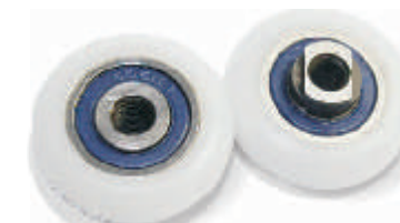
KT1600581 Mode:6001ZZ Steel Type: Stainless Steel/ GCr15 Chrome Steel Plastic Coat: POM/Nylon Size: 12x47 × 16.3mm
